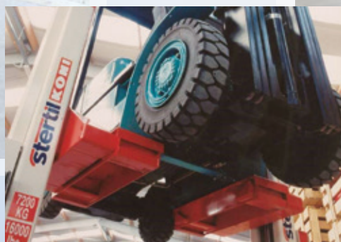
View of Four-Wheel Forklift Adapter Kit undercarriage
